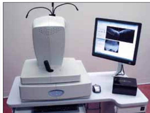
Figure 8d. Spectral domain OCT
